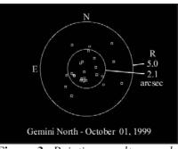
**Figure 3:** Pointing results revealing better than 3 arcseconds rms.
