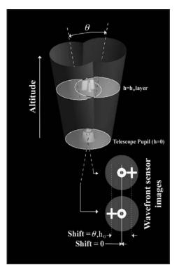
**Figure 1:** Principle of MCAO. The shift of a phase feature signature in the 2-D wave-front sensors is proportional to the altitude of the atmospheric layer which created it. Once reconstructed, the 3-dimensional phase volume is then compensated in a 3-D fashion by using several deformable mirrors conjugated at a range of altitude.
