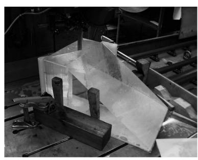
**Figure 1:** Cutting of the large fused silica prism ("immersion prism") at Heraeus. The prism was cut out of a single large rectangular block 612x375x370mm in size and is made out of the highest homogeneity fused silica commercially available (less than 1 part per million variation in the refractive index).
