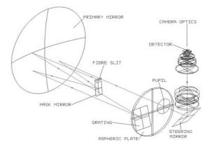
Inside the suppressor the light is dispersed and this dispersed light is reflected off the mask mirror which blocks out the light from the OH lines. If this hardware OH suppression is not required the mask can be replaced by a plain mirror. The cryogenic camera then images the output light from the mask onto the detector.
