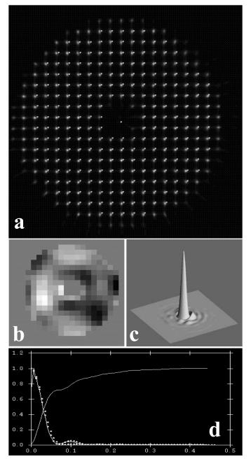
**Figure1 (a-d):** Prime focus wavefront sensor image (a) and data reduction (b-d). Image (a) shows the Shack-Hartman spot pattern of a star with (smaller) reference spots, (b) is an optical path difference map, (c) shows a 3-D point spread function (psf), and (d) is a plot of encircled energy vs. diameter in arcseconds.
