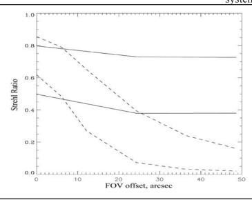
**Figure 2:** J (lower curves) and K (upper curves) Strehl ratio versus off-axis angle for Natural Guide Star systems (dashed line) and for a MCAO system using 5 LGSs, 4 NGSs and 3 deformable mirrors (solid line). Both are 12x12 subapertures Shack-Hartmann systems. This case was run for a zero degree zenith angle, under median seeing conditions, for a typical Cerro Pachón turbulence profile.
