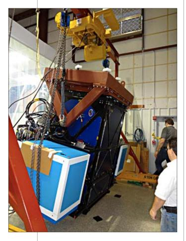
First, GPI was mounted on the flexure rig, then tilted and hung vertically, to simulate the effects of gravity on the instrument, which changes when the telescope points to different parts of the sky (figure 5). Next, GPI went into a cold room and was exposed to the large range of temperatures that will occur at Gemini South.
