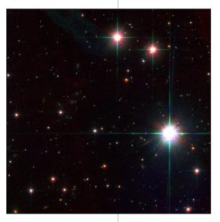
takes images that have been reduced with the Gemini Image Reduction and Analysis Facility package for GSAOI and aligns them by matching sources with the aid of a lookup table that maps the instrument's static distortion. Stacking is then performed with bad pixel rejection and, if desired, inverse-variance weighting. The
